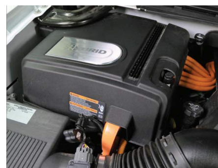
Fig. 42- Inversor / Convertidor NFPA-HEV-EV-Safety-Training-Student-Manual-1.0
